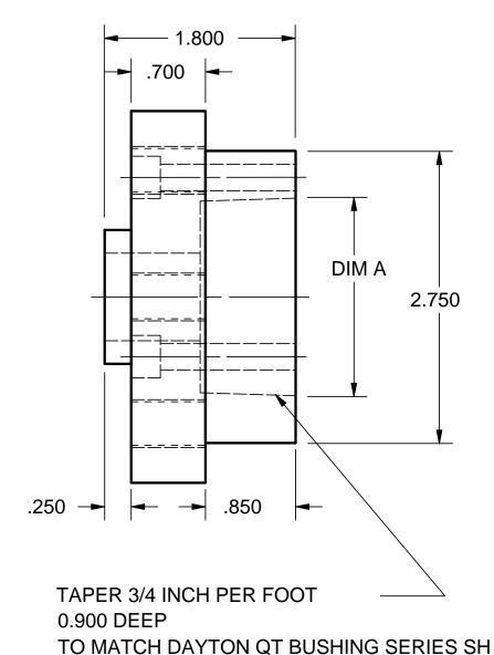
DIM A TO ALLOW BUSHING TO INSERT WITHIN 1/8 TO 3/16
